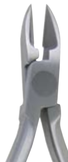
74-107L Micro-Mini Pin & Ligature Cuts soft wire pins and ligature wire up to .012" (.30 mm); Slim design for hard to access areas
