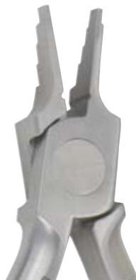
74-319 Nance For forming loops in four lengths - 3, 4, 5 and 6 mm; Groove at base aids in closing loops. Wire capacity .022"
