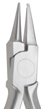
74-305 Light Wire Bird Beak with Groove For forming precise loops in light wires up to .020" (.51 mm). The groove in the tip allows for duplicating loops
