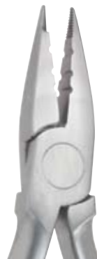
74-301 Jarabak For light wire bending; Grooves assist with precise bending and closing of loops. Serrated surface grips wire up to .02" (.51 mm)
